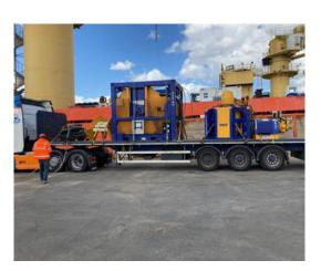
Rotech Subsea were contracted to assist with cable de-burial operations on an offshore wind farm. Rotech provided the RS2 Controlled Flow Excavator (CFE) equipment spread to carry out cable de-burial and Joint de-burial ops.
