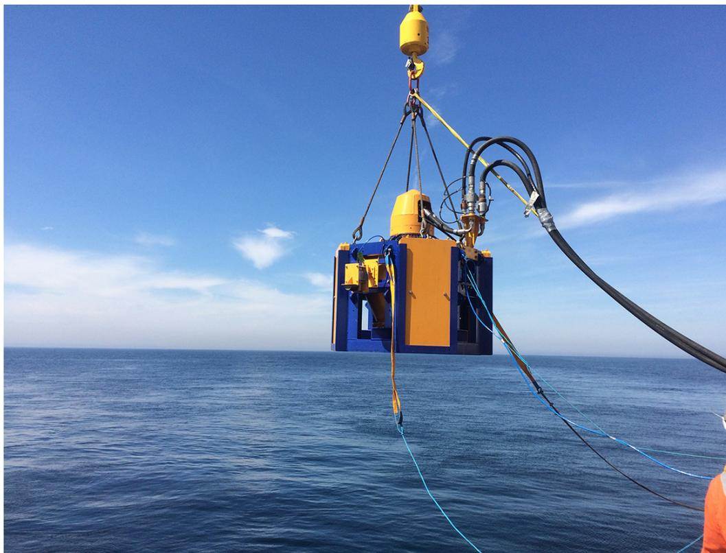
**Rotech Subsea** were contracted by **Prysmian Group** on 2 separate occasions (Q2 & Q3) to provide the RS2 CFE tool for the de-burial of a subsea cable. This allowed Prysmian to access the cable for repair which was followed by post lay trenching of the 180mm cable. Operations were carried out at the Western Link Project.
