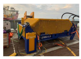
Rotech Subsea were contracted to assist with cable de-burial, post-lay and remedial trenching operations on an offshore wind farm offshore Taiwan. Rotech provided the TRS1LD Controlled Flow Excavator (CFE) equipment spread to carry out this scope.
