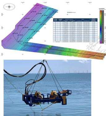
**Rotech Subsea** were contracted by **Jan De Nul** to provide the TRS1LD Jet Trenching tool to carry out Post-Lay Trenching works on Changua Offshore Windfarm, Taiwan. The scope of work consisted of burying a total of 21 cables (4 Export, 17 Array) to client specification of 2.0m DoL. The project will be completed in 2 phases.
