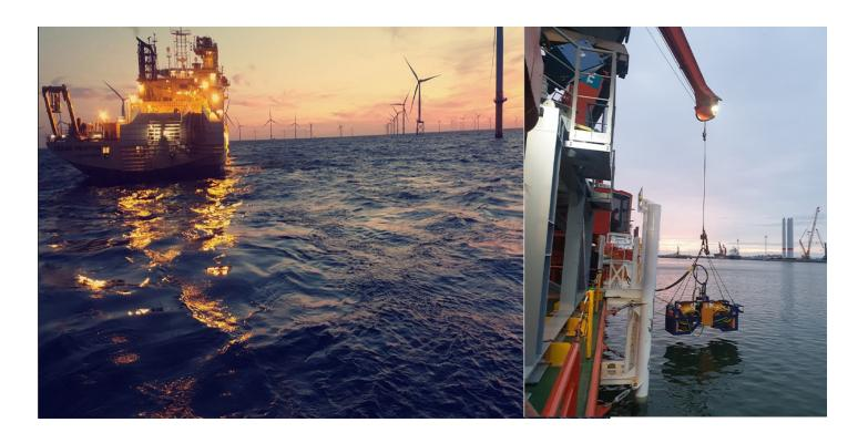
**Rotech Subsea** were contracted by **Jan De Nul** to provide the TRS1 CFE tool to carry out cable de-burial. Following the installation of the new subsea cable, Rotech Subsea post-lay trenched to Jan De Nul's specification of 1.7m Depth Of Burial. The scope of work was carried out at Bokrum Rifgrund OWF, offshore Germany.
