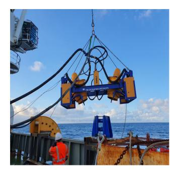
**Rotech Subsea** were contracted by **Boskalis** to provide the TRS2 CFE tool for Pipeline Deburial and Rock Dump dispersal. The scope of work consisted of dispersing 70m of rock reaching a depth of 1.2m. The Rock Dump material reached **12 inches** in diameter.
