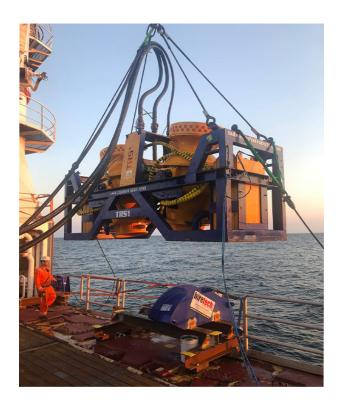
**Rotech Subsea** were contracted by **Deepocean** to carry out pipeline de-burial works on the Thames-Bacton 24" gas pipeline. The scope of work consisted of de-burying approximately 80m of pipeline and to carry out 3 spot excavations at different locations to allow access for cutting. The pipeline was buried **0.7m TOP** from the mean seabed level.
