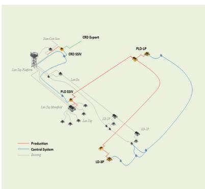
**Rotech Subsea** were contracted to **Subsea 7** for Umbilical post trenching. This was completed between Lan Tay platform and Phong Lan Dai SSIV with a route length of approximately 4.14km.
