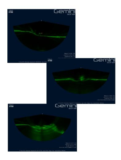
**Rotech Subsea** were contracted by **Subsea 7** to carry out Sandwave Peak Shaving operations. Peak shaving was completed along the 16-inch flowline between well PLD-1P and Lat Tay Manifold approximately 20.73Km. Umbilical post trenching was completed between Lan Tay platform and Phong Lan Dai SSIV with a route length approximately 4.14Km. The water depth in the area was 192m.
